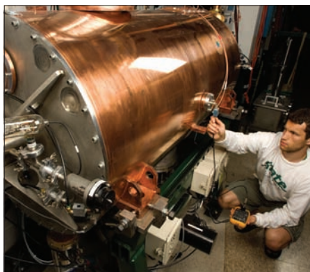
NSCL doctoral student Josh Stoker checks the radio frequency fragment separator, which provides additional capacity to study neutron-deficient nuclei. The separator, initially proposed by NSCL users in 2004, is available for experiments following the lab's reconfiguration. (Courtesy NSCL.)
